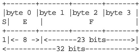
Just as the most and least significant bytes of a number are 0 and 3, the most and least significant bits of a single-precision floating-point number are 0 and 31. The beginning bit (and most significant bit) offsets of S, E, and F are 0, 1, and 9, respectively. Note that these numbers refer to the mathematical positions of the bits, and NOT to their actual physical locations (which vary from medium to medium).
