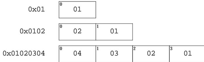
Encoding `ELFDATA2MSB` specifies 2's complement values, with the most significant byte occupying the lowest address.
