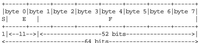
Just as the most and least significant bytes of a number are 0 and 3, the most and least significant bits of a double-precision floating-point number are 0 and 63. The beginning bit (and most significant bit) offsets of S, E, and F are 0, 1, and 12, respectively. Note that these numbers refer to the mathematical positions of the bits, and NOT to their actual physical locations (which vary from medium to medium).
