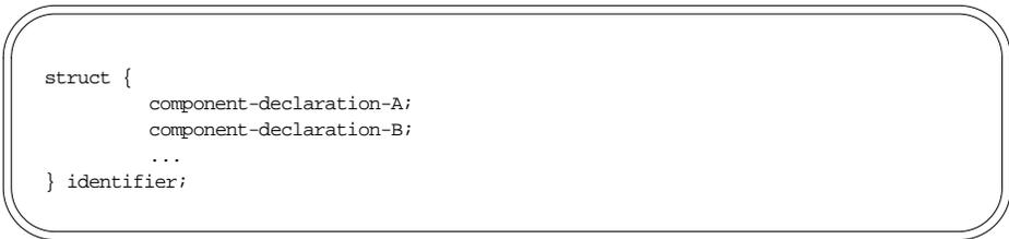
The components of the structure are encoded in the order of their declaration in the structure. Each component's size is a multiple of four bytes, though the components may be different sizes.
